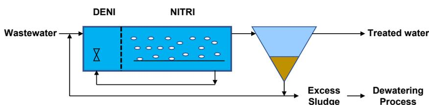
Figure 2: Schematic of wastewater treatment process
