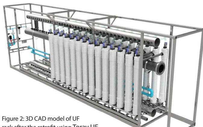
Figure 2: 3D CAD model of UF rack after the retrofit using Toray UF showing additional room for expansion. Image courtesy of WesTech Engineering, Inc.
