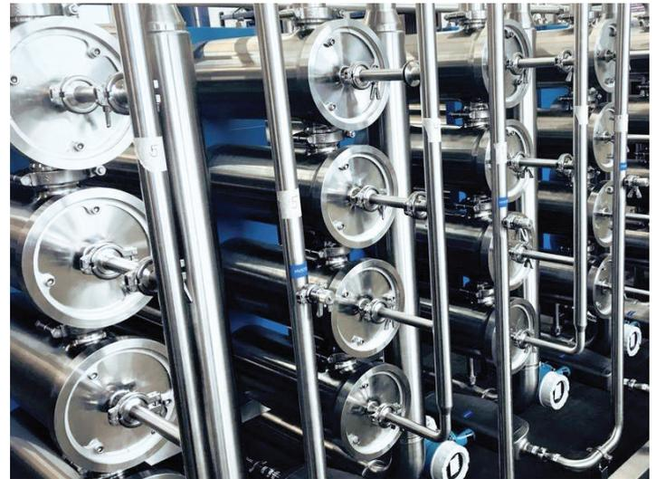
Figure 1: Heat sanitisable RO system. Image source MMS AG Urdorf Switzerland
