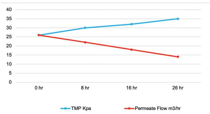
Figure 1: TMP and permeate flow of the capillary UF system
