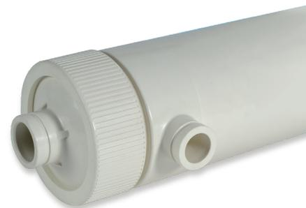
The ultrafiltration (UF) system was comprised of two trains, each with 28 modules, using inside-out capillary type UF membrane modules to produce a permeate flow of 60 to 80 m<sup>3</sup>/hr. The UF membrane material was a polyethersulfone (PES) with a nominal pore size of 0.025 μm.
