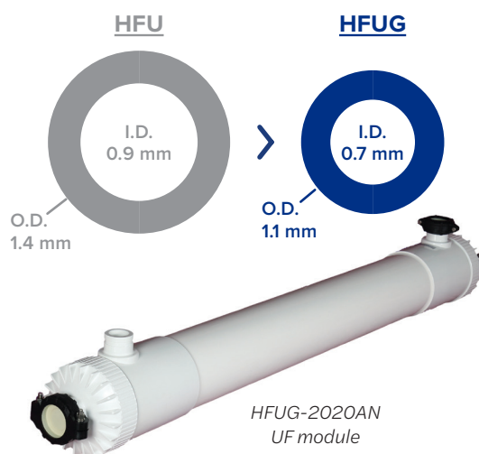
Figure 3: UF hollow-fiber diameter comparison
