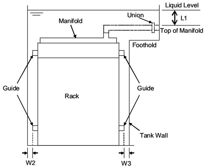
Fig. 7 Rack Layout in Membrane Submerged Tank (side view)
