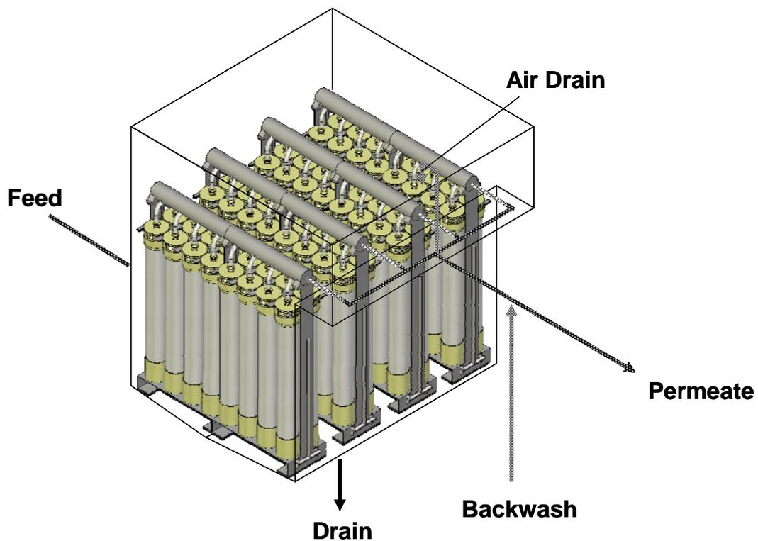
Fig. 4 Image of “Rack” (4 units of R16 Model are submerged in tank)
