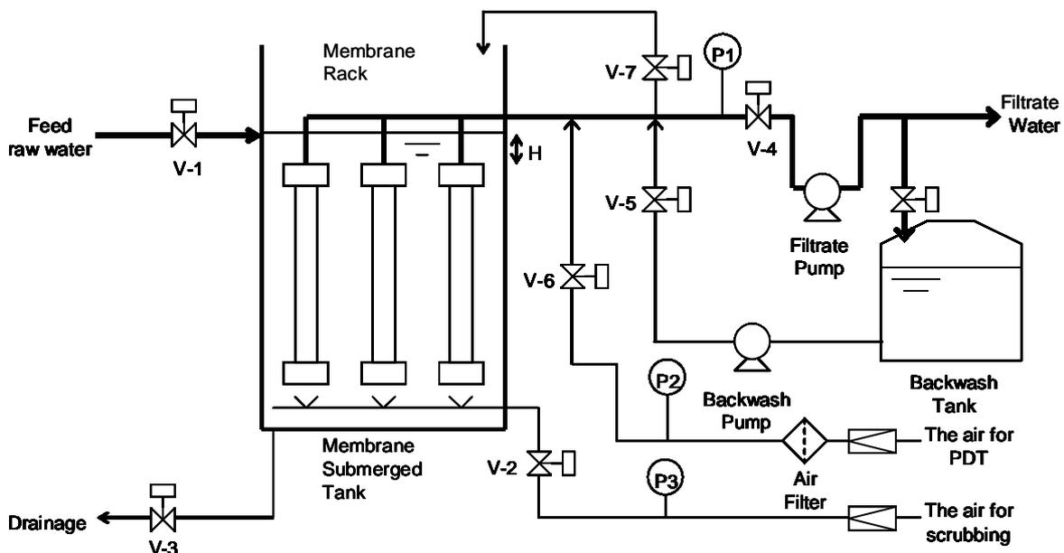
Fig. 16 Flow diagram for the PDT
