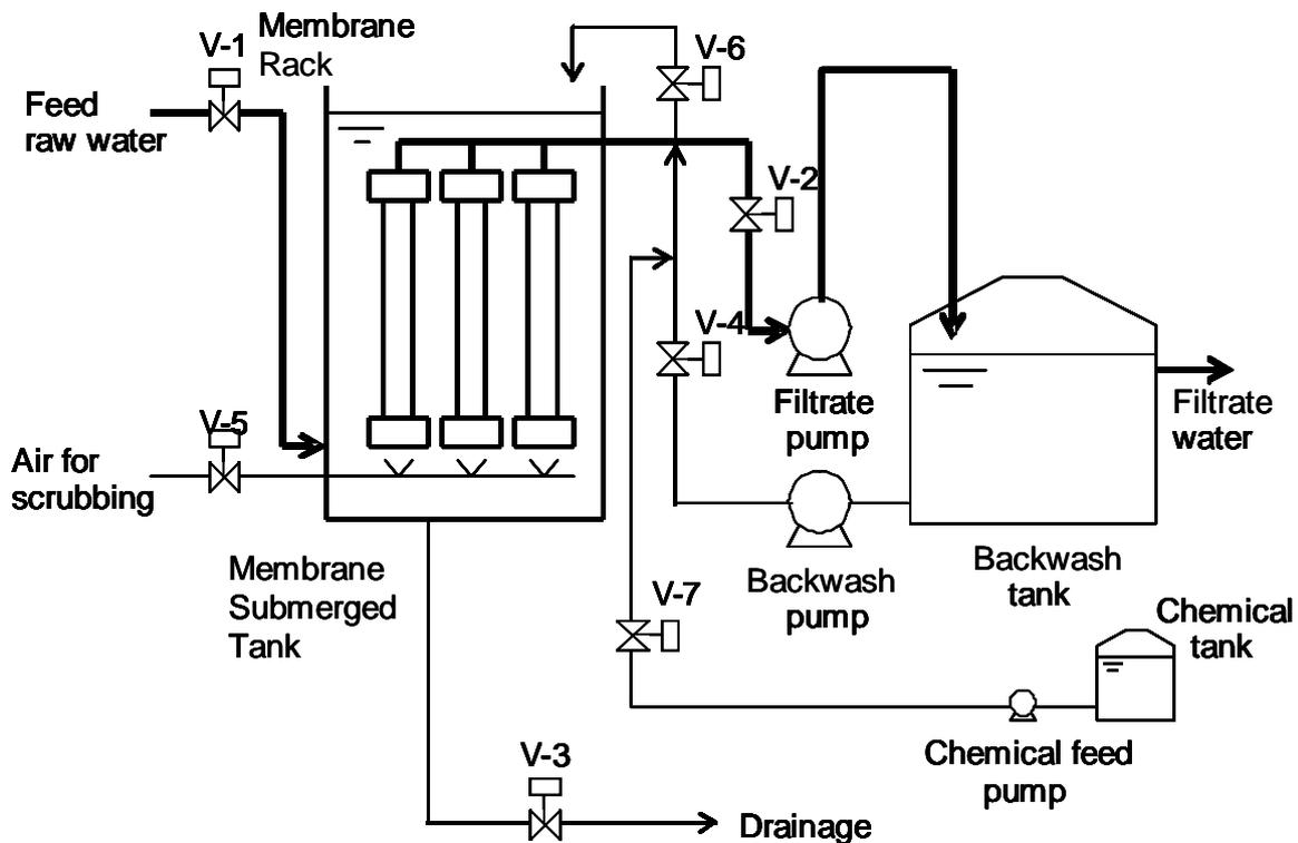
Fig. 10 Flow diagram for filtration
