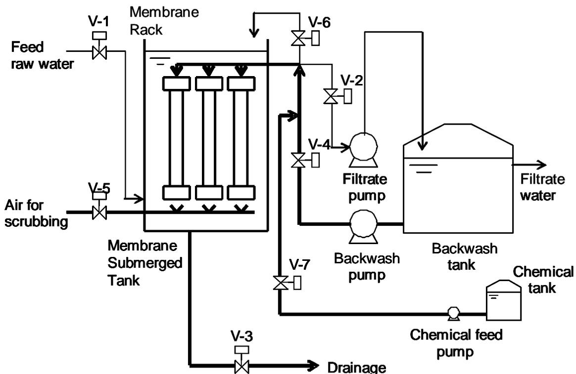
Fig. 11 Flow diagram for backwash and air-scrubbing
