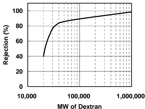
Fig. 2 Molecular weight cut off (MWCO) of the HSU membrane
