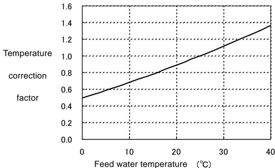
Fig. 15 Temperature correction factor (TCF)
