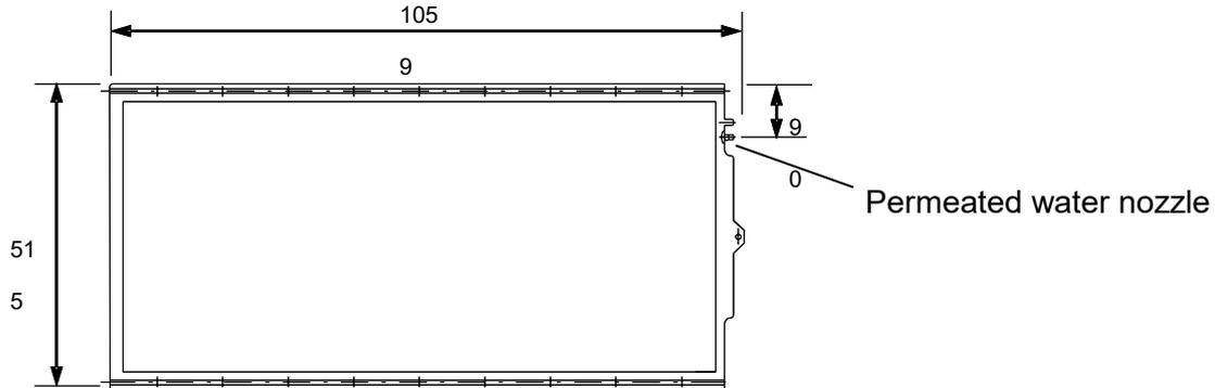
**Fig.III-1 Appearance of Element (unit: mm)**
