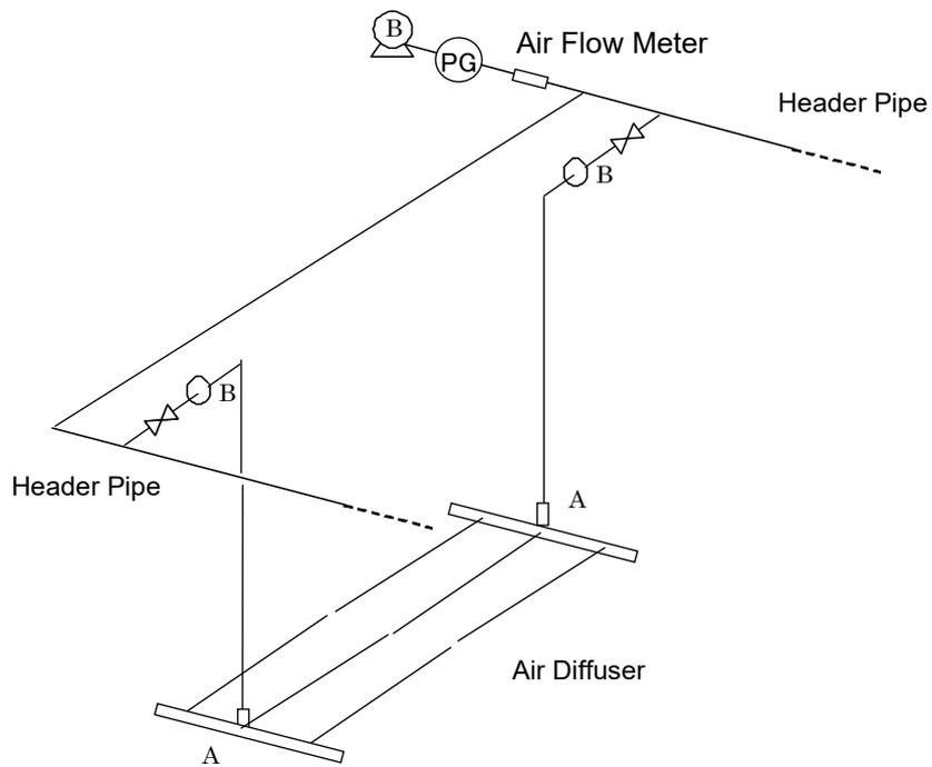
**Fig.IV-11 Example of Piping to Air Diffusers for TMR090-100S (Installation of Multiple Units)**
