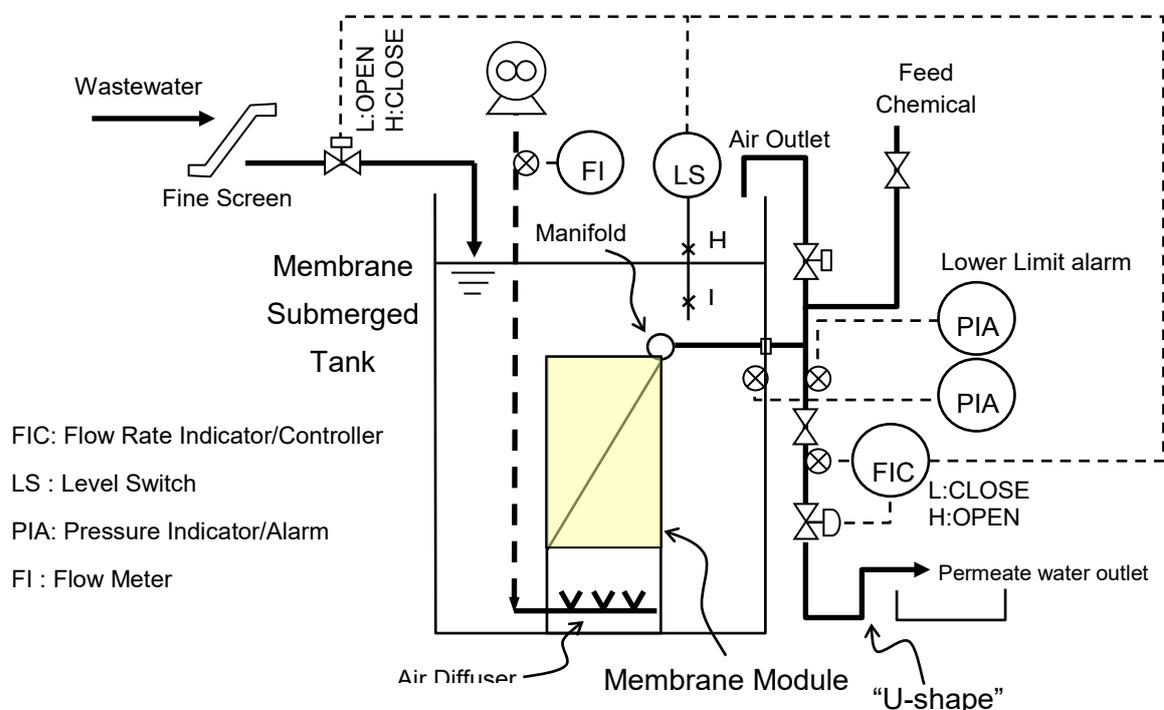
**Fig. IV-2 Schematic Flow Diagram for Gravity Filtration**
