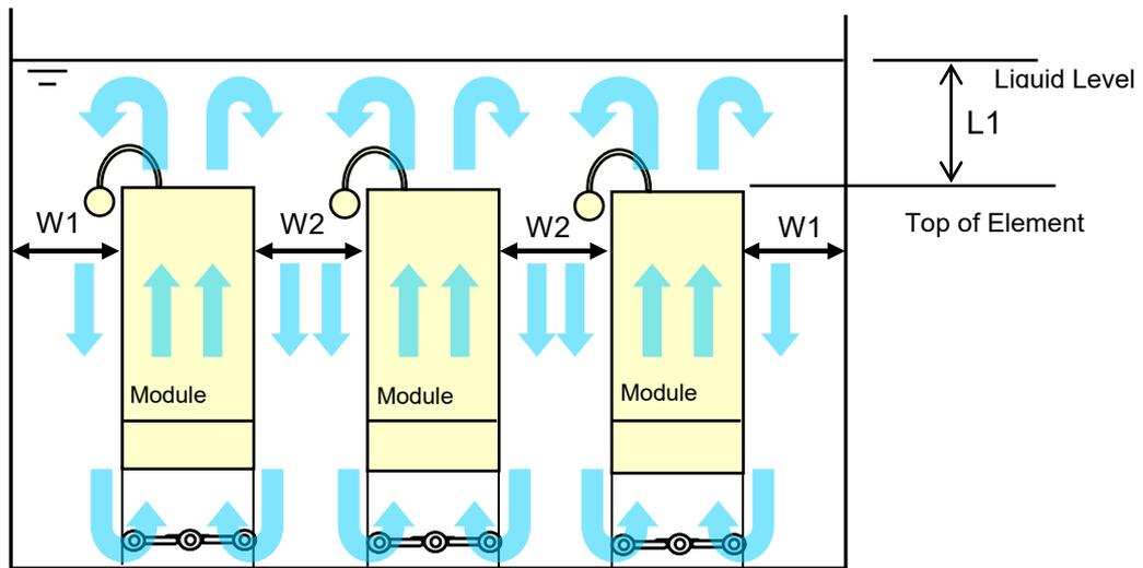
**Fig.IV-5a Membrane Module Layout in Membrane Submerged Tank (side view)**
