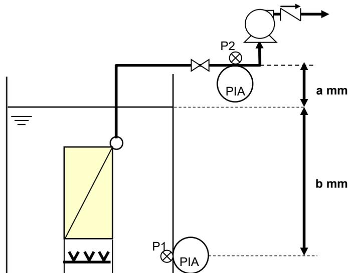
**Fig.IV-4 Differential Pressure Measurement & Calculation**
