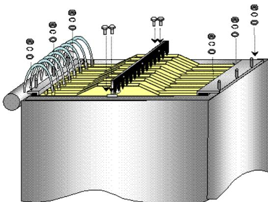
(3) Install element fixing brackets on the element block. After installation, check that comb gaskets are touching elements flat.
