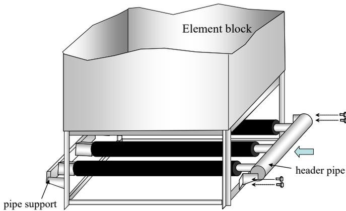
(5) Fit the header pipes to the aeration block while fixing air diffusers on the pipe supports.
