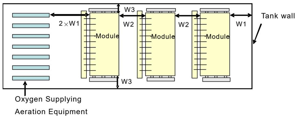
**Fig.IV-8 Membrane Module Layout in Membrane Submerged Tank with other aeration equipment (top view)**
