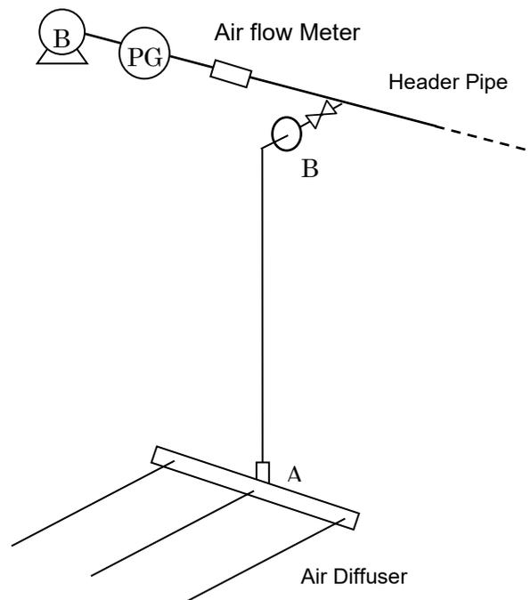
**Fig.IV-9 Example of Piping to Air diffusers for TMR090-050S**
