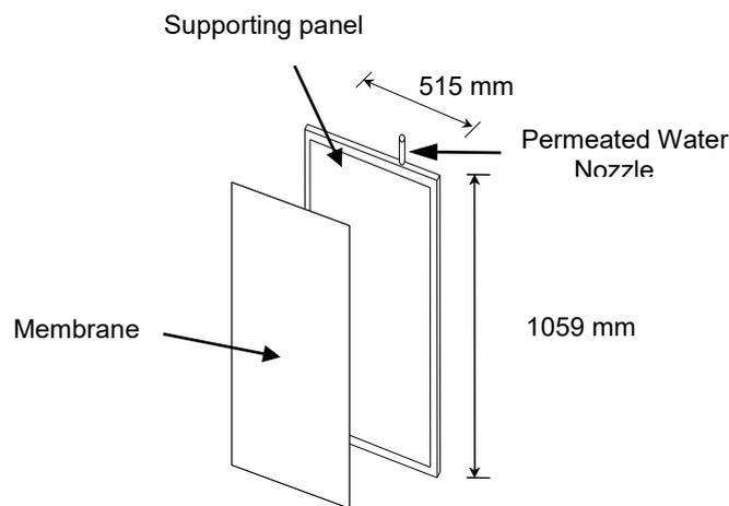
**Fig. I-4 Structure of Element**
