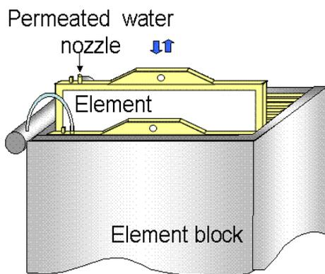
(2) Remove three element fixing brackets from the element block according to the element fixing bracket replacement procedure above.
