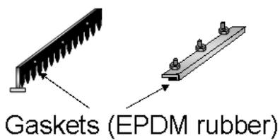
(2) Replace the comb gaskets from each bracket. The gaskets consist of several parts according to the type of module. Detailed information will be provided separately.
