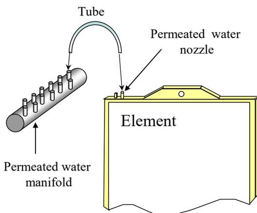
(6) Fit tubes straight down to element nozzles and manifold nozzles.
