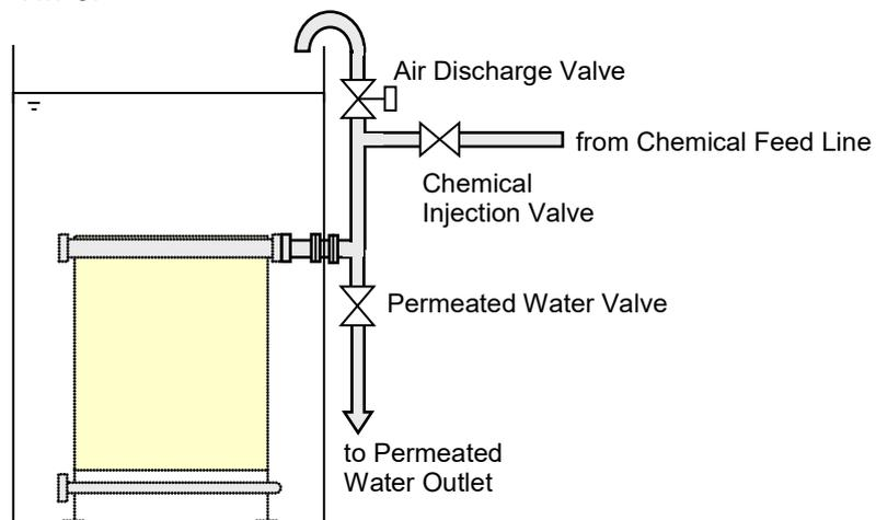
**Fig.IV-12 Downward Piping from Membrane Submerged Tank**
