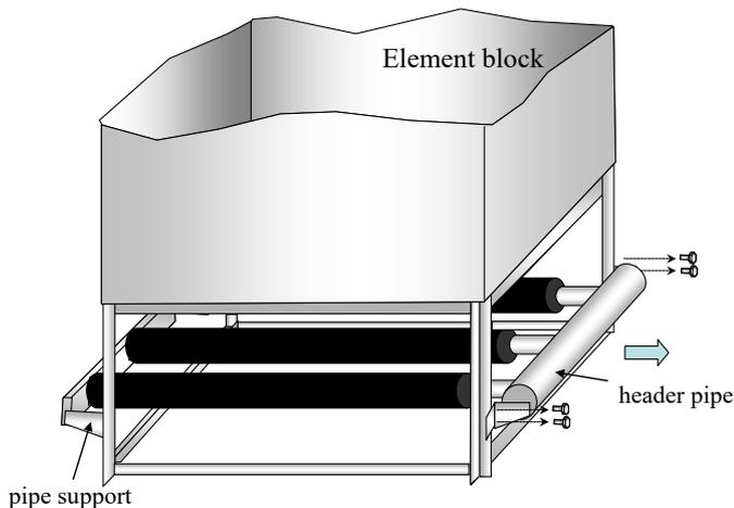
(1) Disjoint the header pipe from the aeration block.
