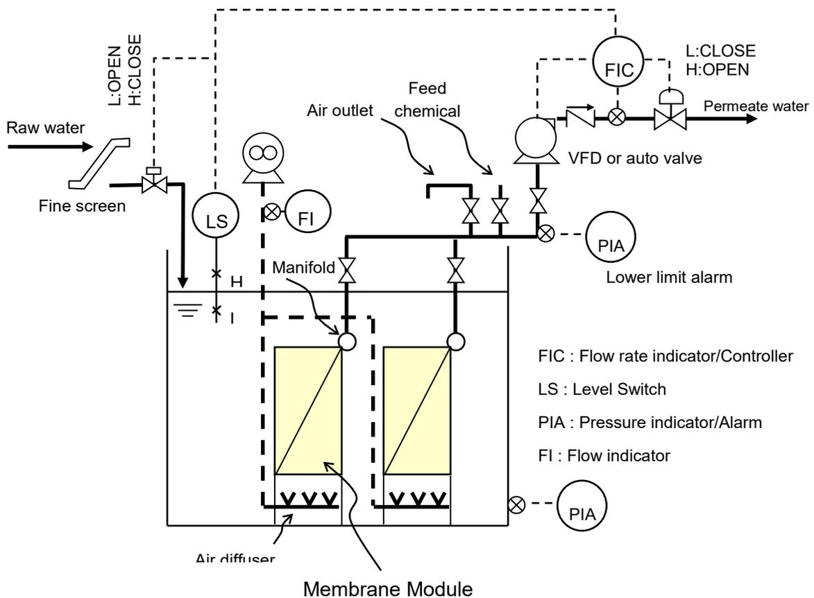
**Fig.IV-3 Schematic Flow Diagram for Pump Suction Operation**
