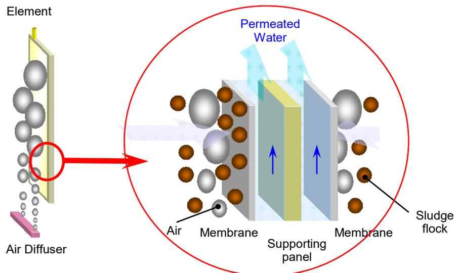
**Fig. I-5 Filtration Principle of Activated Sludge**
