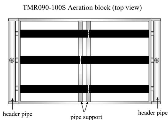
In case of TMR090-100S, since two different lengths of the rubber diffusers are to be handled, please take enough care to joint air diffusers considering the position of
