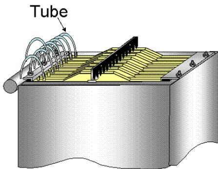
(1) Pull the permeate tubes, which are to be replaced, out from element nozzles and manifold nozzles.
