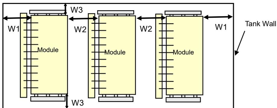
**Fig.IV-5b Membrane Module Layout in Membrane Submerged Tank (top view)**
