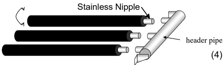
(4) Joint the new air diffusers to the header pipes. Please use the pipe wrench to tighten the joint (Don't fasten tight by grabbing the rubber part of the diffuser). Please make sure that the surface of the rubber part having no holes (slits) must face upward or downward (The surface on which stainless clamps are fixed must face upward or downward).
