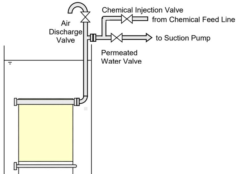
**Fig.IV-13 Upward Piping from Membrane Submerged Tank**
