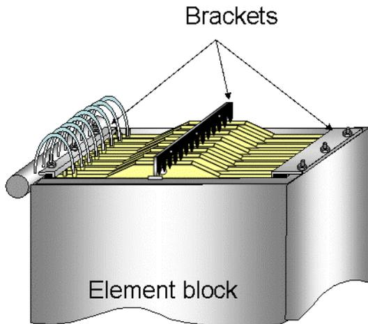
(1) Remove the three element fixing brackets from the element block (one center bracket and two side brackets).
