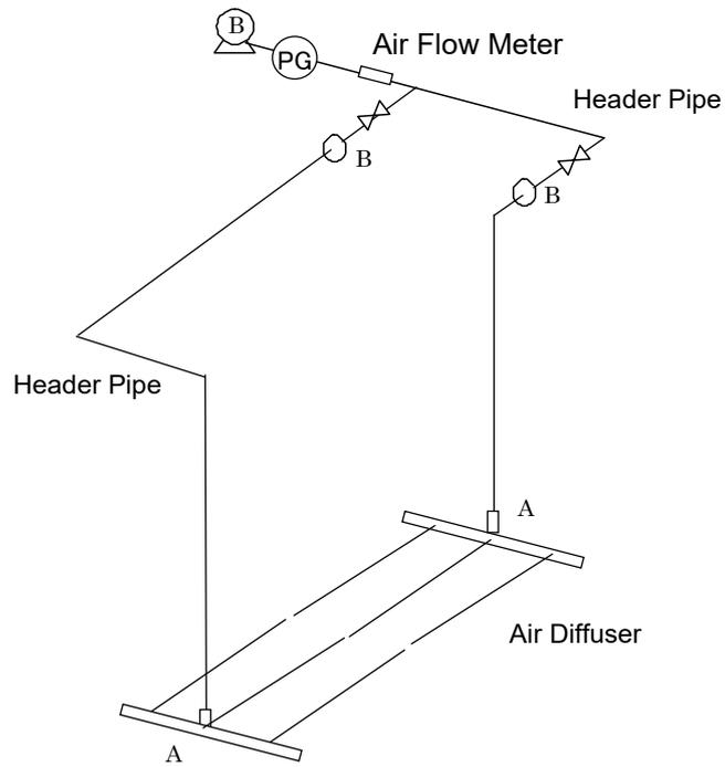
**Fig.IV-10 Example of Piping to Air diffusers for TMR090-100S (Installation of One Unit)**
