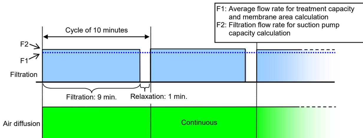
**Fig.IV-1 Recommended Time Cycle for Intermittent Filtration**
