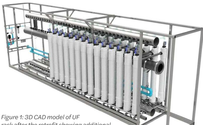
Figure 1: 3D CAD model of UF rack after the retrofit showing additional room for installation. Image courtesy of WesTech Engineering, Inc.
