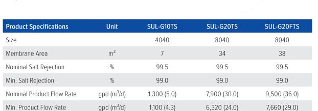
**Test Conditions**: Feed water pressure 110 psi (0.75 MPa); Feed water temperature 25°C (77 °F); Feed water concentration 500 mg/L as NaCl; Brine flow rate 20 l/min (5.3 gpm) for SUL-G10TS, 80 l/min (21.1 gpm) for SUL-G20TS and SUL-G20FTS; Feed water pH 6.5
