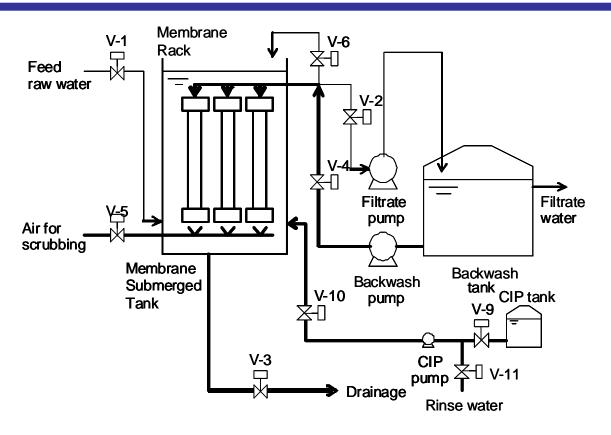
Fig. 18 Flow diagram for chemical cleaning
