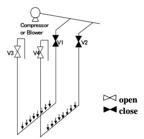
Fig.12 Condition when air scrubbing F
