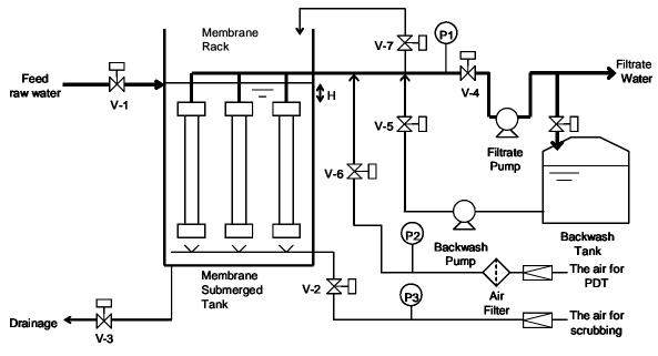
Fig. 16 Flow diagram for the PDT
