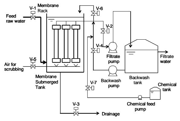
Fig. 9 Typical example of piping
