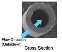
Fig. 1 Cross section picture of Toray PVDF hollow fiber
