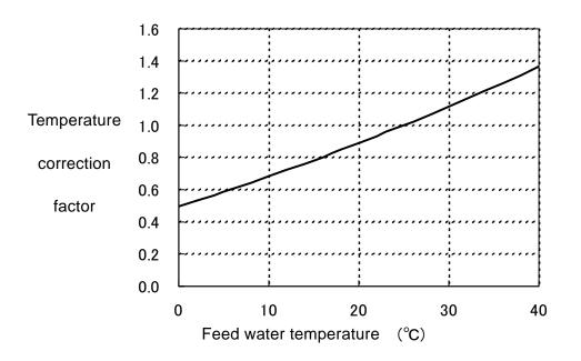
Fig. 15 Temperature correction factor (TCF)
