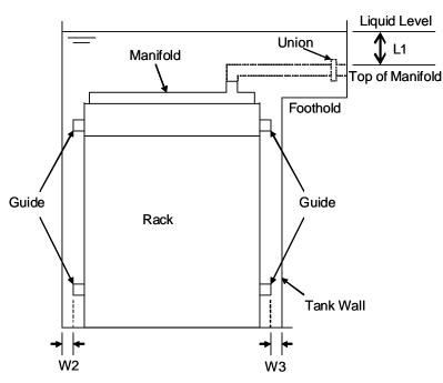
Fig. 7 Rack Layout in Membrane Submerged Tank (side view)
