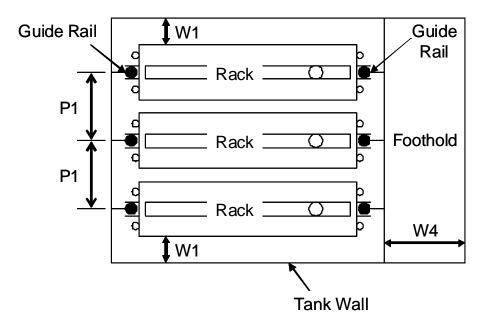
Fig. 8 Rack Layout in Membrane Submerged Tank (top view)
