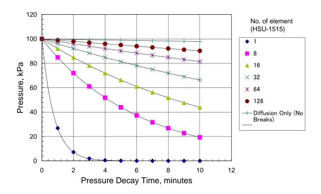
Fig. 17 HSU-1515 pressure decay rates with one broken membrane fiber (calculated)
