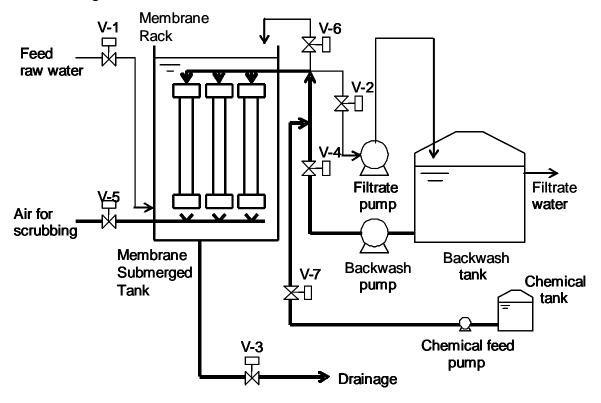
Fig. 11 Flow diagram for backwash and air-scrubbing
