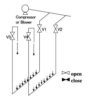
Fig. 14 Condition when cleaning process
