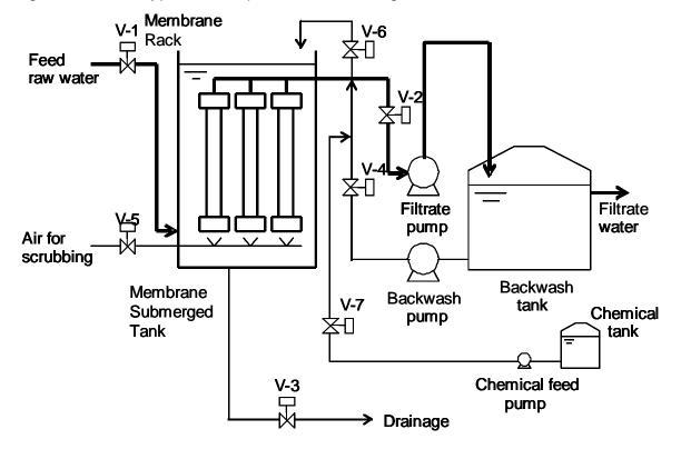
Fig. 10 shows a typical example of the flow diagram for filtration.
