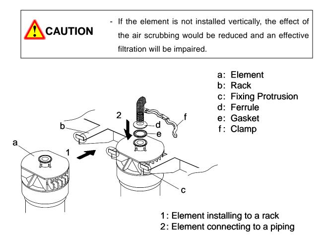
Fig. 6 Installation of Element in Membrane Rack
